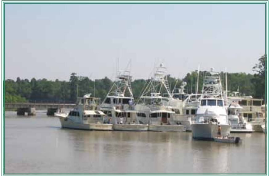
A strategy that worked beautifully: Boats from Dog River Marina in Alabama were taken up the Tenn-Tom Waterway by professional captains. Using multiple anchors and lines to shore, all of the boats survived with no damage. Boats that remained at the marina weren't so fortunate.
