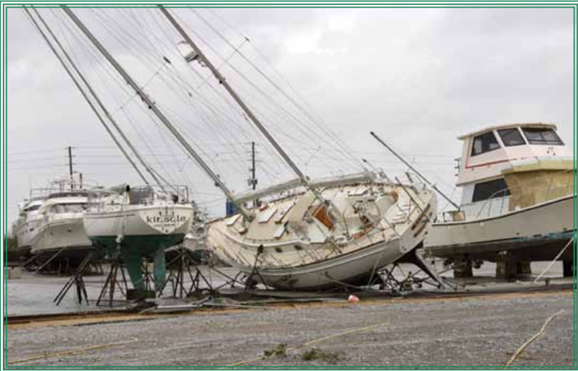
The boat above was blown over, despite being secured to earth anchors, by a combination of windage (masts) and too much stretch in the nylon lines (note the slack in the lines to the boat on the left). Jack stands on the leeward side buckled.
